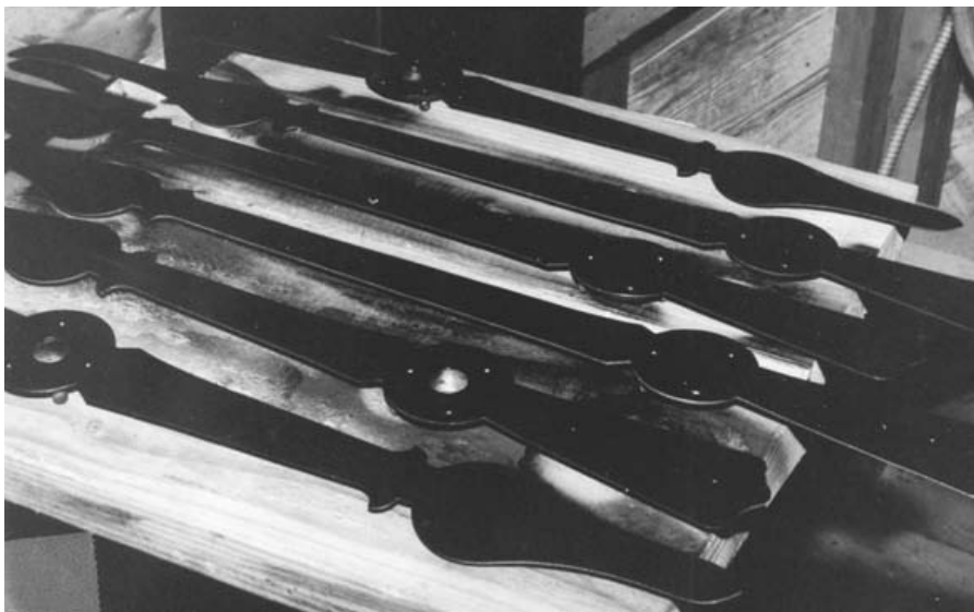
Figure 8. Repainted tower clock hands.
