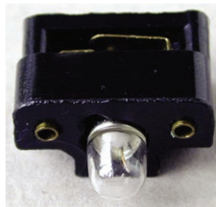
Figure 5. The lamp module removed from the base.
