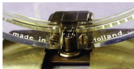
Figure 6. Rear of clock showing brass screws that attach the outer dial ring.
