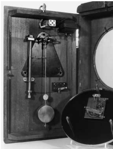
Figure 22, above. Jamin-Zenith clock without power reserve, mid 20s. The dilation wire is in the tube seen on the left. It acts on the pendulum through an elastic lever and a traction wire at the bottom. Contacts are on the top of the pendulum. This constitutes a sort of thermic motor working under 4V AC, independent from the dial, which is, again, just an oscillation meter.
