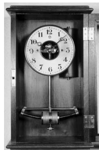
Figure 2, above. One-second pendulum clock of the Hipp type signed Favarger & Cie, about 1910. The dial is an oscillation meter linked to the pendulum by a fork and gathering system.
