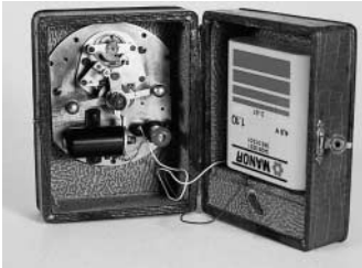
Figure 8. Small Swiss travel clock signed Cosmos, using the cheap version of the Reform movement, based on patents from 1928 and 1929. It has a spiral balance with a spring giving a power reserve of some three minutes to the going train. When the spring reserve is almost exhausted, a small arm linked to the barrel closes the contact and the electro-magnet gives a kick to an inertia arm with two balls at the ends. This winds up the spring with a pawl and ratchet and at the same time interrupts the contact. This movement is more commonly found in its high quality version, with 15 jewels and Breguet hairspring.
