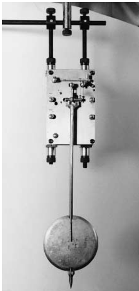
Figure 14. Aron movement of 1884, signed G. Becker, Freiburg in Schlesien. The electro-magnet is on the left and acts on the pendulum through an arm when the contact closes. The arm is linked to the pendulum and carries a pawl in order to index the wheel train. Interestingly, the dial has a minute sub-dial graduated in number of vibrations (80) and not seconds.
