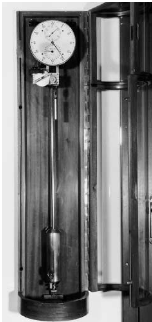
Figure 9. Wall clock with Ferramo balance movement, made by T. Baeurle & Sons, Sankt Georgen, Black Forest, using a Ferraris motor for the winding power. The main advantage of this motor is that it is silent, a quality that not all electric clocks can claim to have!
