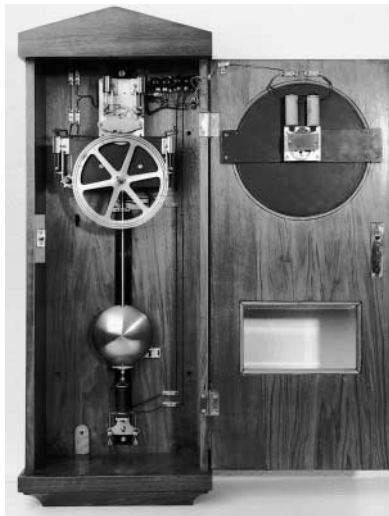
Figure 23, above. Favag master clock with 2/3s pendulum. Late 1920s. Fitted with additional module consisting of a 24-hour contact wheel for actuating signals that are adjustable in five-minute intervals.
