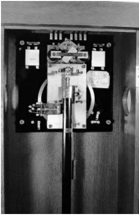
Figure 7. An EZ clock of the 1930s (EZ = Elektro-Zeit, later becoming T&N = Telefonbau & Normalzeit). In contrast to the common pawl and ratchet rewind system found in many electrically rewound clocks, the electro-magnetic system in the EZ clock is composed of a two-pole armature that is pivoted to rotate through about 25° into alignment with the magnetic field when the contact is closed and returns to its resting position under the force of a weak spring when the contact is opened. This sudden rotational energy is transferred through the surface of the contact to a large flywheel that winds up a small weight, sufficient for driving the anchor escapement and pendulum for a few minutes until the process is repeated. This electro-magnetic “motor rewind unit” is a discreet module from which the pendulum also hangs, and the conventional anchor movement comprises another easily removable module (not in the picture) that counts the pendulum beats and displays the time on a dial. These two units are linked together by a helical spring through which energy is transferred with maintaining power. The clock illustrated has, in addition, two wheel trains linked by a differential, one for the time and one for the secondary clocks contact, revolving once per minute of a half-rotation and reversing the polarity at the same time.
