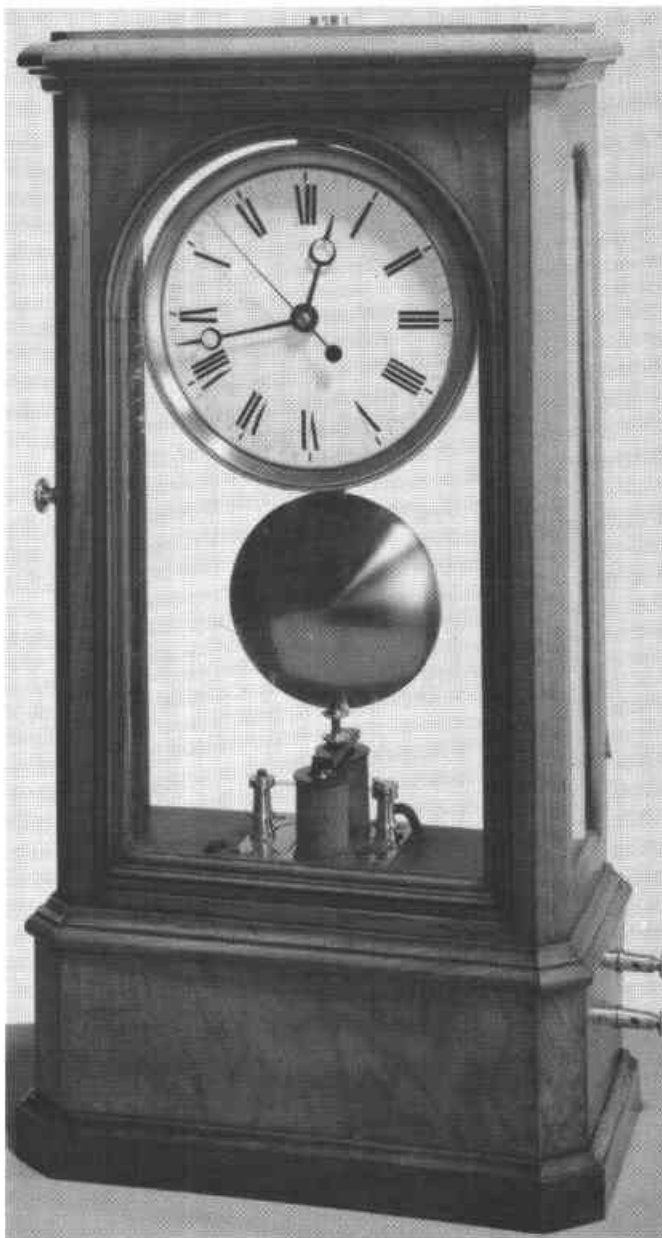
Figure 6. An early example of a Hipp toggle electric clock made at Neuchâtel, Switzerland, the only reliable electric clock of the mid-nineteenth century.
