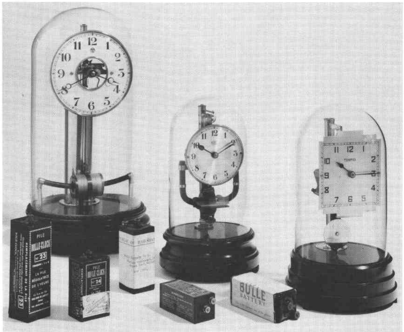
Figure 13. Left and middle—the two most commonly found Bulle clocks, right—a cheaper version of the Bulle manufactured by Tempex, the base is of bakelite. In the foreground are samples of the driving batteries.
