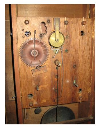
The access holes in the corners of the movement are small. 'Small' is defined as up to and including 9/16" diameter.
